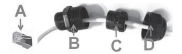
(3) Install an RJ45 connector on the unterminated end of the Ethernet cable using an Ethernet cable installation tool. Wrap waterproof materials around the Ethernet cable between part B (split gasket) and C (grommet).
