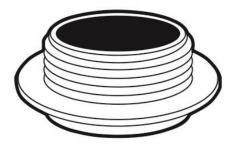
Connect the network cable, optical fiber jumper, and DC power cable to the access point after they pass through the corresponding waterproof plugs to ensure waterproof.
