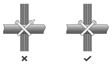
• When cables need to be bent, bind them first but do not tie cable ties within the bend. Otherwise, considerable stress may be generated in cables, breaking cable cores, as shown in Figure 7-6.
