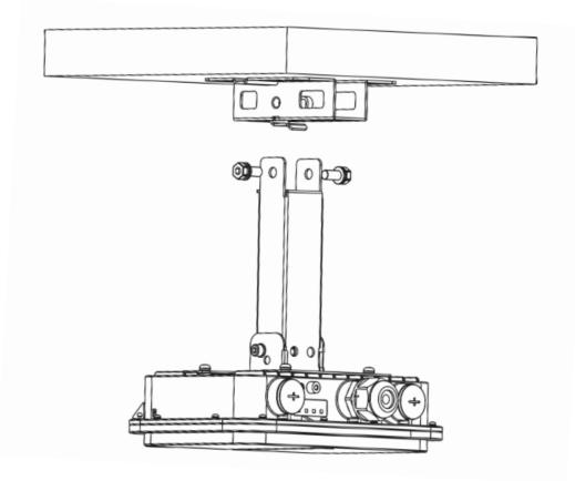
(5) Use two M8 screws to secure the mounting arm to the mounting bracket.
