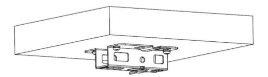
(2) Loosen the two M6 screws on the mounting plate assembly to remove the mounting arm. Rotate the mounting arm by 90 degrees clockwise until it is upright. Tighten two M6 screws to secure the mounting arm to the mounting plate.
