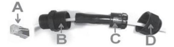
(4) Insert the RJ45 connector into the Ethernet/PoE port of the access point, and tighten the cable gland assembly in sequence of part B, C and D to complete the installation.
