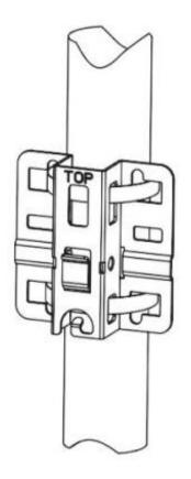
Horizontal pole mounting: Secure the mounting bracket to a horizontal pole by threading two hose clamps through the square holes of the mounting bracket. Keep the part of the bracket noted by **TOP** on top.
