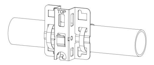
(3) Position the mounting arm on the mounting bracket with its two holes aligned to the screw holes on the mounting bracket.
