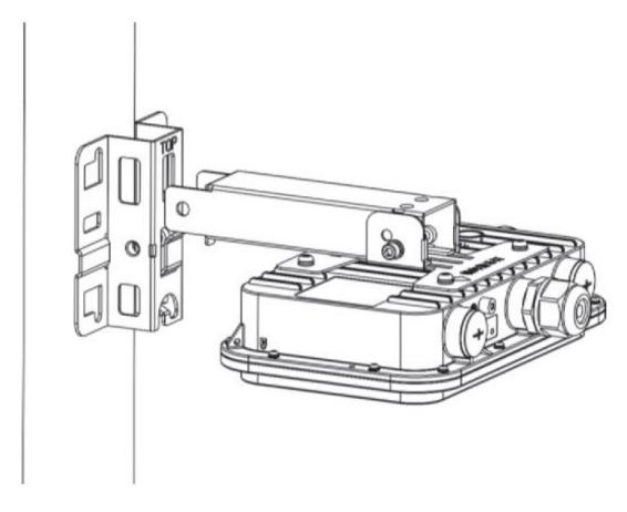
(4) Use two M8 screws to secure the mounting arm to the mounting bracket.
