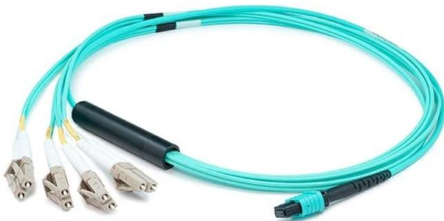
Parallel optical technologies such as 40G SR4/eSR4 and 100G SR4 optical transceivers can also split into four separate optical streams to connect to 10G SR or 25G SR/eSR optics on the opposite end of the link using fiber breakout cables.
