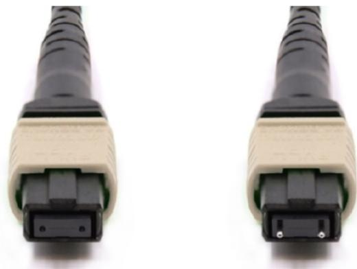
The 40G SR4 and 100G SR4 MPO transceiver modules use only cables with female MPO connectors, which have guide holes in the end face of the MPO connector (the transceiver has guide pins within the MPO receptacle).
