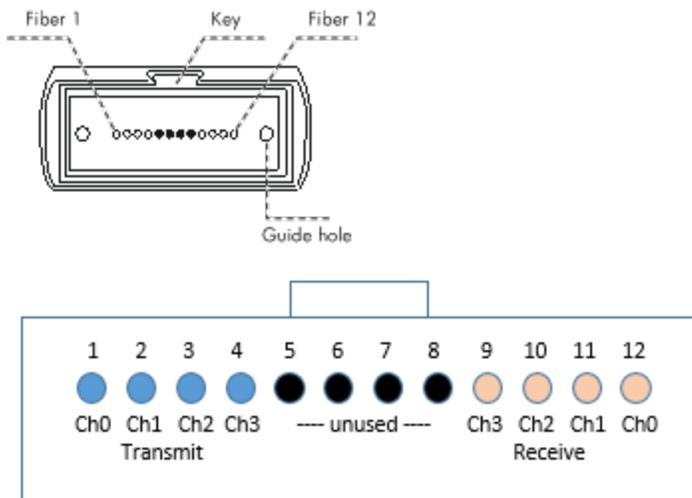
MPO transceivers typically use four channels to communicate. These channels are assigned using the outer eight fibers (the center four are unused).
